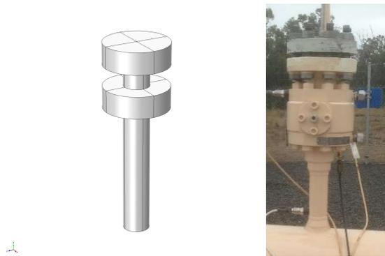
**FIGURE 4 - EXAMPLE CASE; TWO FLANGES ON A SMALL-BORE CONNECTION. MANY SUCH REAL-WORLD EXAMPLES EXISTS**
