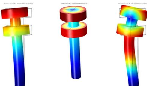
**FIGURE 5 - EXAMPLE CASE; FIRST NATURAL FREQUENCIES AND SHAPES**
