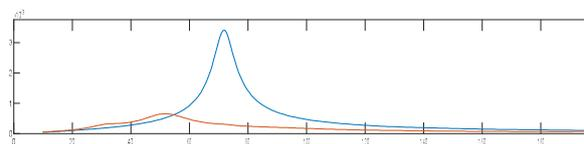
**FIGURE 7 - THEORETICAL VIBRATION RESPONSE WITH (RED) AND WITHOUT (BLUE) A MOMENTUM TMD**
